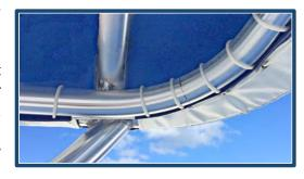
design and determined it is actually stronger than the typical upper-lower bar arrangement because it has 2 horizontal pieces welded to the cross-members instead of just 1. The design did create a bit more work on Steve's end because now the corners were compound curves requiring more planning, cutting, and sewing.
